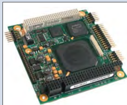
PC/104-Plus boards like the Kontron MOPSIcdLX PC/104-Plus often don't require active or passive cooling.
